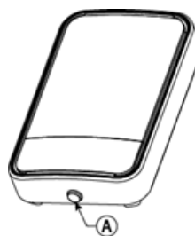
A. SR-740 PG2 can be recognized outwardly by its red screw cap. B. Wall
