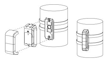
Figure 8: Curved surface mounting
