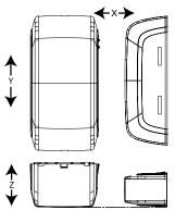
Figure 10: Range coverage directions (with perpendicular magnet)
