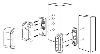
Figure 7: Flat surface mounting
