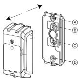
Figure 6: Device and bracket separation
